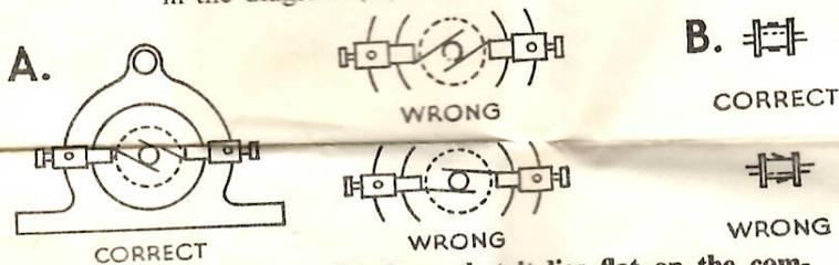
**Be careful to insert brush so that it lies flat on the commutator—not twisted at an angle (B).**
