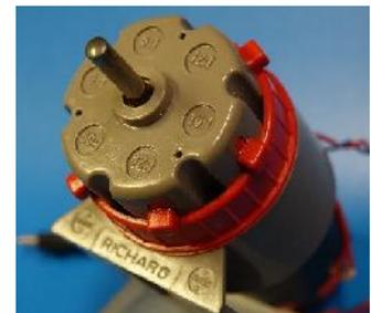
This Marx Richard Gear Motor had several unique features such as a forward, off & reverse switch and a built in gearbox with 6 gear ratios. The red ring on the gear case could be turned to the selected ratio setting a speed suitable for the vehicle it was installed in. The forward, off and reverse functions of this motor would be remotely controlled by the actuator above . This motor required a 6 volt battery.
