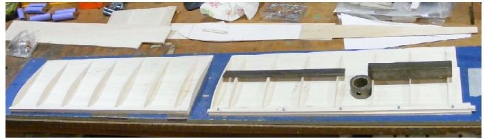
Ribs added to lower wing skins
