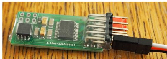
You may, of course prefer to make your own leads, possibly by soldering together two leads cut from old broken servos. If you are intending to power your motor / actuator via this cable (and the pulser's link) make sure that the cable has thick enough wires to carry the necessary current.
