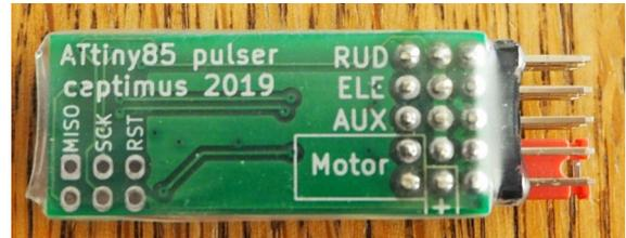
The pulser can operate motors / actuators that work at voltages up to 15V, and at currents up to 2.4A (average) or 6.4A (peak).
