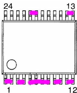
Don't worry if you notice apparent 'solder shorts' on the TB6612FNG chip (the larger of the two chips on the board). Some pins are intentionally connected via the tracks on the PCB: when soldering, the solder tends to bridge across adjacent connected pins. This is nothing to worry about and, if anything, probably helps a little by lowering the resistance between pins that are already linked anyway. The image at the left shows which pins are linked.
