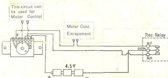
With this wiring, motor control is done with Relay Counter Contact.
