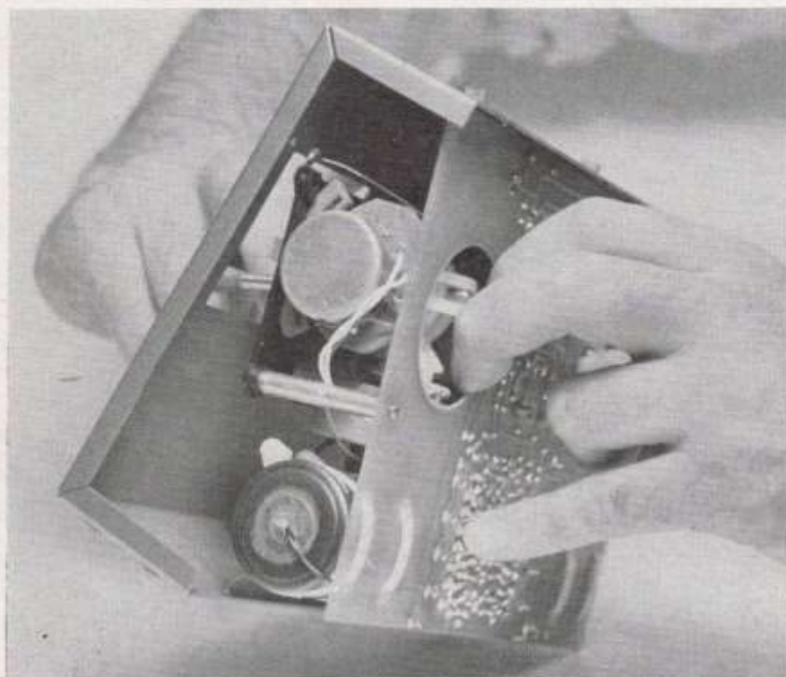
Fig. 10. The assembly of the Tx p.c. to case, not how auxiliary control levers are engaged first. After fitting, all that remains is a final check on the tuning of L.1 and L.2.
