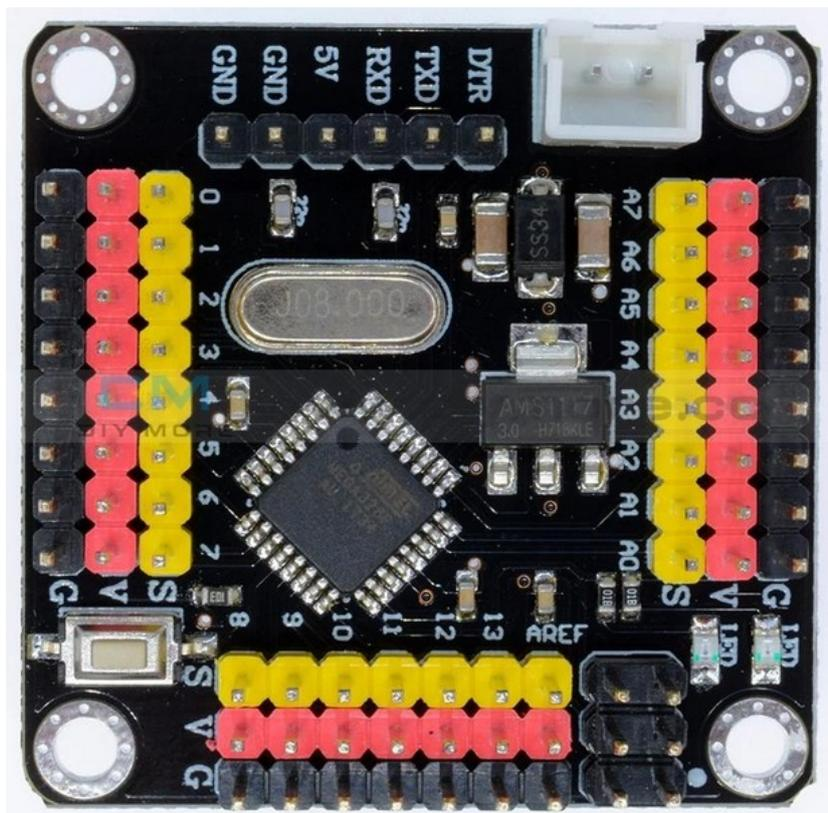
2. Use a 5V Arduino, but power it from your own regulated 3.3V supply into its VCC pin (not Vin/Raw). You can use a 16 MHz Arduino – yes it will almost certainly work okay at 3.3V.
