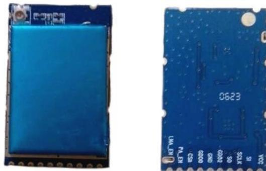
The larger modules, example pictured above, can connect to a ‘proper’ antenna (often not supplied with the module, but you can buy the antennas separately, or salvage one from an old R/C transmitter or a WiFi router). Don’t power up the larger modules unless an antenna is connected. These modules, equipped with a good antenna, have a transmitting range equaling or surpassing that of most commercial R/C transmitters.
