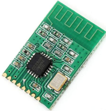
The one pictured above the connections are (left to right): 1:GND 2:(3.3V) 3: SI (MOSI) 4:SCK 5:SO (MISO) 6:no connection 7:no connection 8:CS (most likely Arduino pin 10, but see below).
