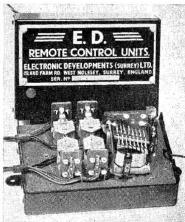
Above: Receiver with top removed. Note that eight reeds are installed on this four channel unit though four only in use. Below: Underside of the unit.
