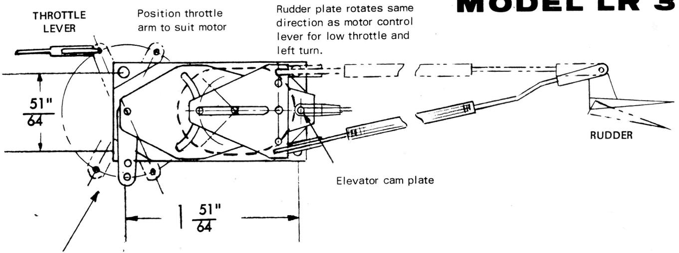
Slip clutch permits movement to any position.
