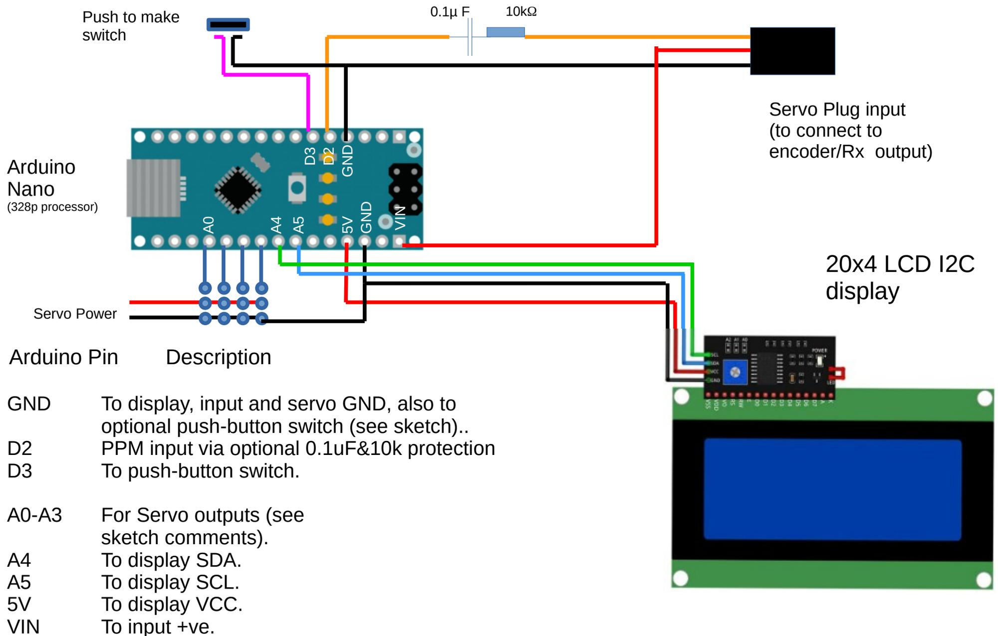
PPM/PWM Tester, 16ch display and servo output – Nov 2022. Sketch: PPMTesterLCD20x4I2C\_16ch.ino
