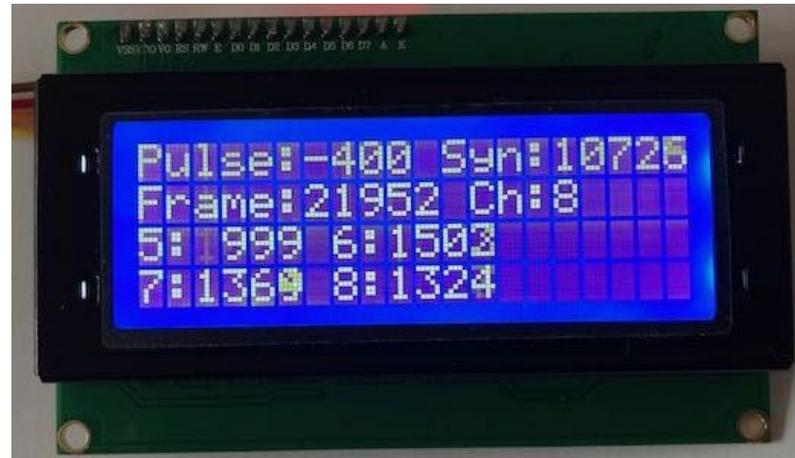
With I2C display connection only 4 outputs are available for servos. The push button is used to toggle between screens, for the first screen only channels 1-4 are output. For second screen onward, the 4 outputs match the display. A maximum of 16 channels is defined, but see Phil\_G's original post for caveats.
