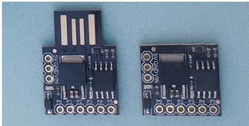
As supplied the board has two schottky diodes D3 and D4 which interfere with the expected operation of port pins P3 & P4. The diodes are easily removed by gently prising with a small screwdriver:
