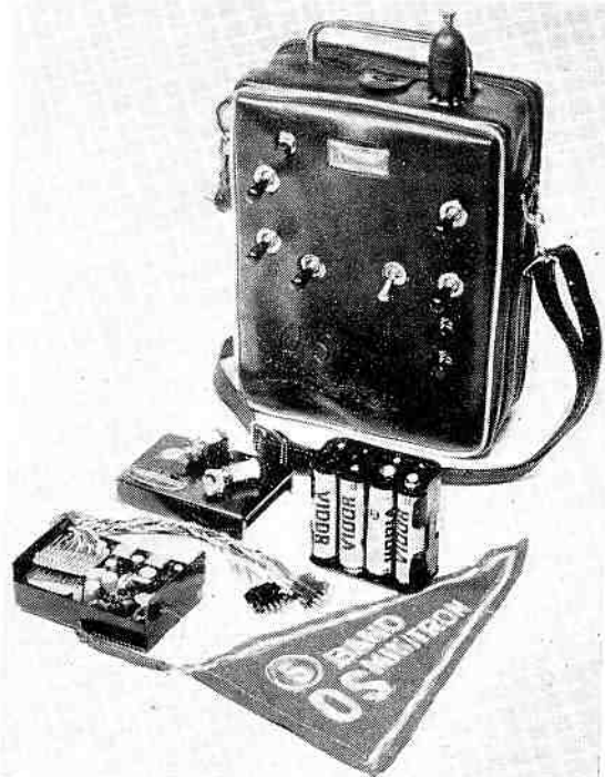
The complete O.S. Minitron 12 channel system as supplied direct from Japan, arrived in complete working order. System is provided with transmitter battery box, receiver connectors, switch and jack plug, plus frequency pennant.
