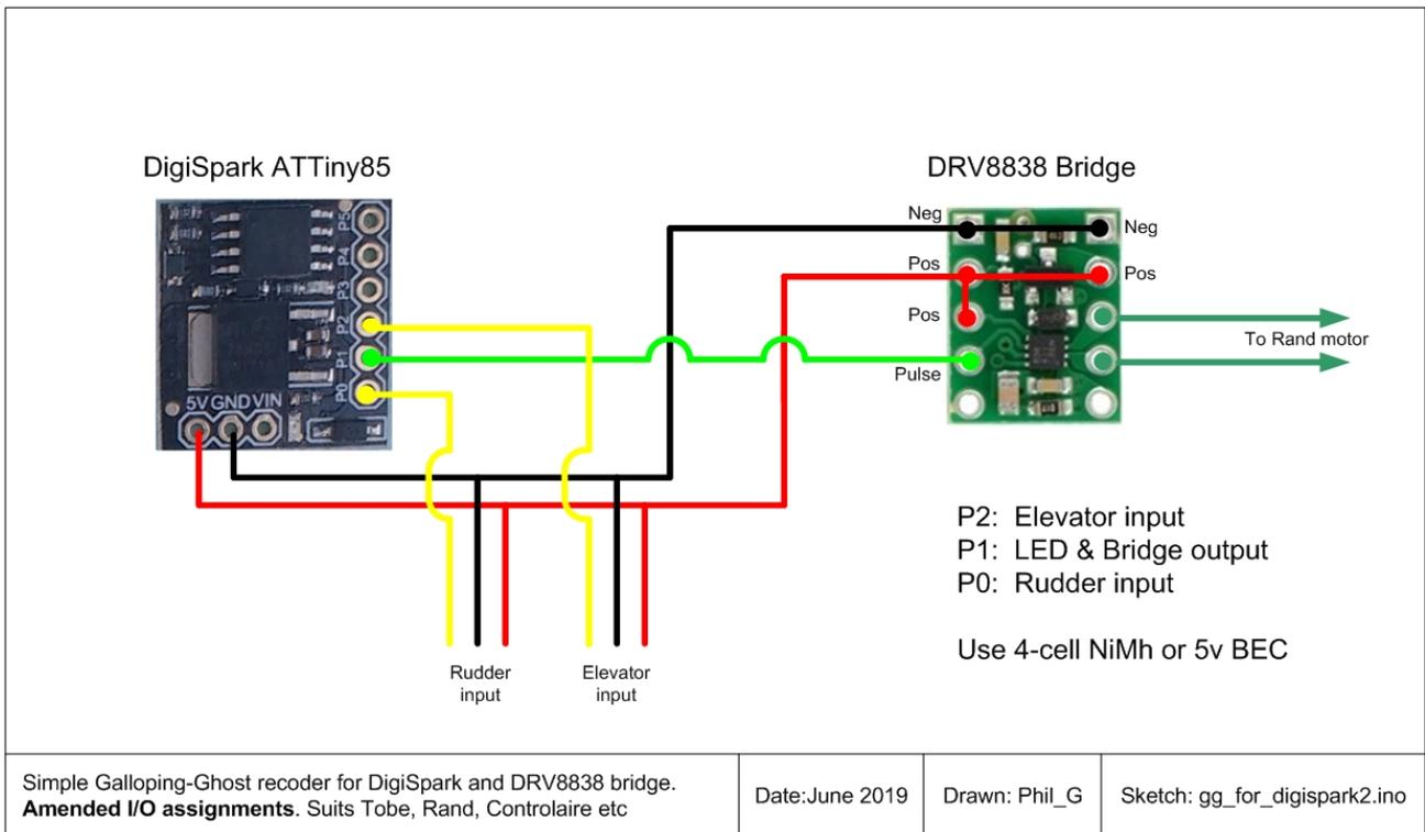
This way the actuator is powered from the receiver supply, but as with the PIC recoder, the actuator can optionally have a **separate battery** if required by chopping the receiver positive supply to pin 9, and providing a new positive from the separate battery. The negatives are common:
