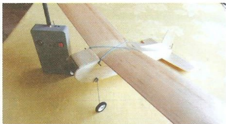
The mighty 'Guided Mite' used a SC escapement together modern 2.4 GHz electronics.
